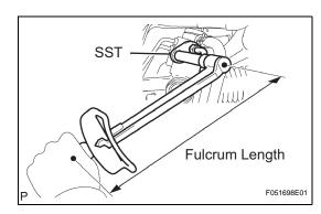
(b) Using SST, tighten the flare nut and connect the pressure feed tube.
